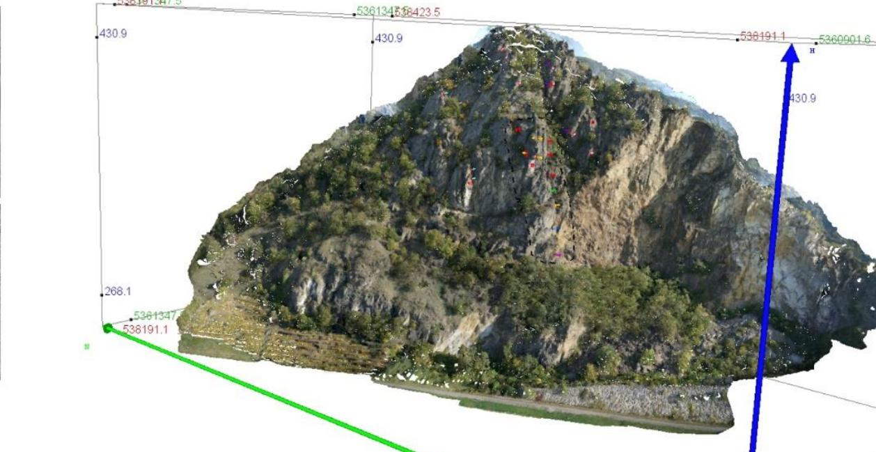
Fig. 4: Structural geological overview mapping by means of a photorealistic 3D model generated using the 3D image measurement system ShapeMatrix-UAV with a Sony A7R camera. (Abb. von Gaich, 2019, Melzner et al., 2019).
