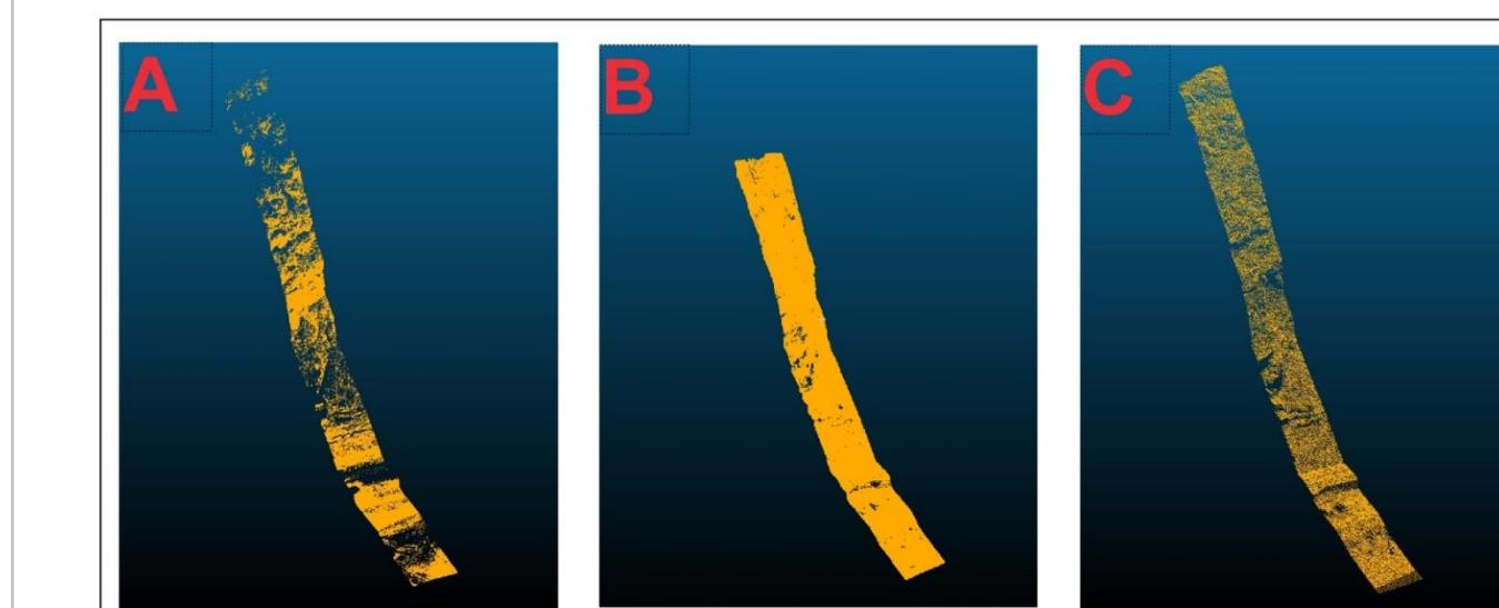
Fig. 5: Structural geological surveys using LIDAR data. Definition of quality criteria of remote sensing data. Coverage of filtered LIDAR data collected by (A) TLS (static), (B) ALS (UAV) and (C) ALS (aircraft) (Melzner and Schwarz, 2019).
