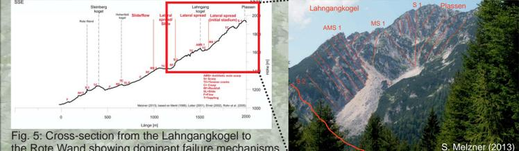
Fig. 5: Cross-section from the Lahngangkogel to the Rote Wand showing dominant failure mechanisms and processes.
