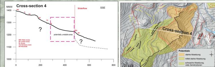
Fig. 6: Mapping of potential unstable areas and selection of cross-section for geoelectric measurements.
