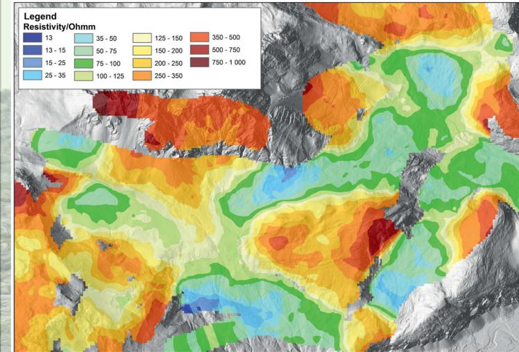
Fig. 4: The pattern of the resistivities shows a good correlation between the different lithological units, which provides lateral delineation and depth up to 70m of these units.
