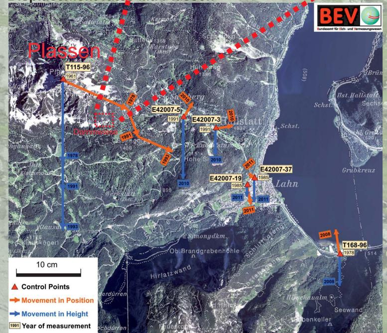
Fig. 10: The point T115-96, near the peak of Mt. Plassen, was measured four times from 1961 to 1993. The analysis of the data shows significant movements of the control points (Source: Department „Control Survey“ of BEV).
