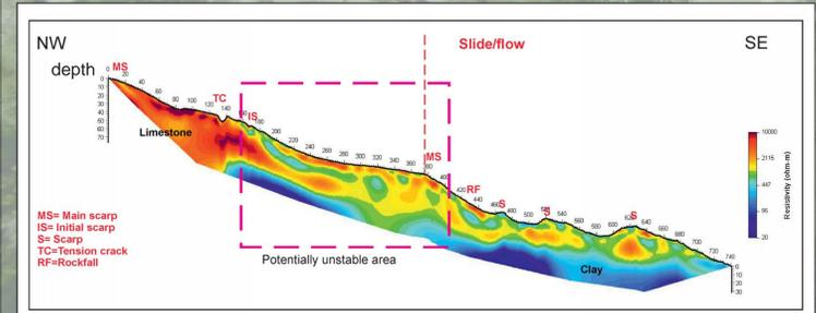
Fig. 7: Geoelectric measurements in a potentially unstable area. Results indicate shear plane which may result in a sliding failure. Orange= limestone; (dark) blue= clay, marl; for location see white line in Figure 6.
