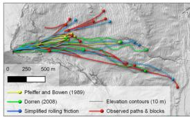
Fig. 6: Sets of five simulated trajectories from three rebound models compared aside the mapped observed rockfall paths shown in red (*Noël et al.*, 2023). Vellow trajectory: Pfeiffer and Bowen (1989) friction; blue trajectory: stnParabel multiple model simulation freeware (Noël 2020); green trajectory: Nockyfor3D v5.2.15 (EcorisQ 2022, Dorren, 2008).
